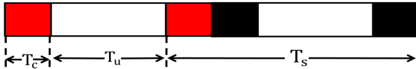
Fig 4.7 The structure of the OFDM symbols
